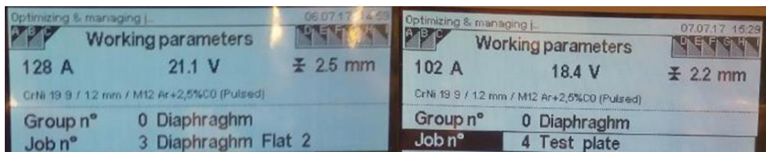
Fig. 5.5 Installation of shims into seal groove and run-in/run-out plates on a both sides of the diaphragm rail (a) , synergic lines (“jobs”) for flat and fillet weld beads (reference) (b).
