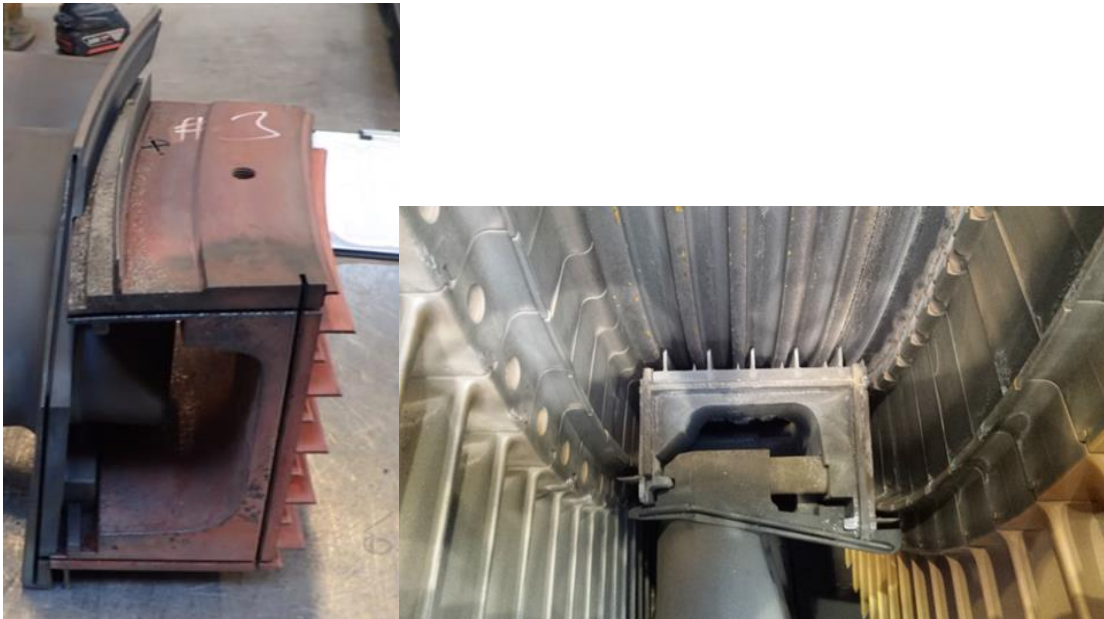
Fig. 5.1 Gas turbine diaphragm (a), Diaphragm rail (b)
